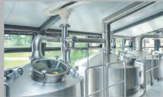
Skid solution for automatic operation (25 hl – 40 hl)
